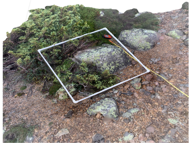
FIGURE 2 A completed digital surface model of a 1-m 2 quadrat on Mt. Guyot, New Hampshire, USA (rendered here in two dimensions). This model was rendered from 40 photos taken with an iPhone 10.
